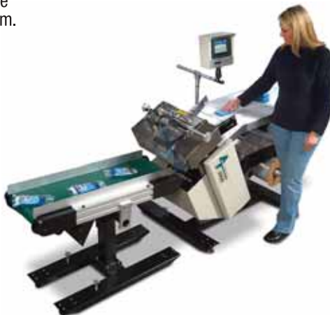
Bulky or lightweight products are difficult to package in a traditional, vertical bagger. Davida manually slides product (sponginess) toward an open bag.
