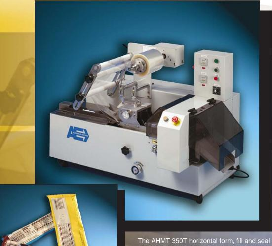
The AHMT 350T horizontal form, fill and seal machine (flow wrapper) is the ideal choice for suppliers of products that must be packaged individually. These products include candies and confections, bakery, electronics, hardware, and medical products.
