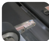
Closing conveyor for smooth product transfer
